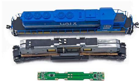
Figure 1: Locomotive with shell and light board removed
