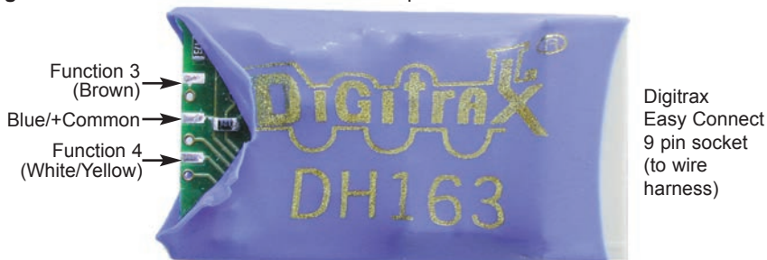
Figure 2. DH163AT Decoder Function Outputs
