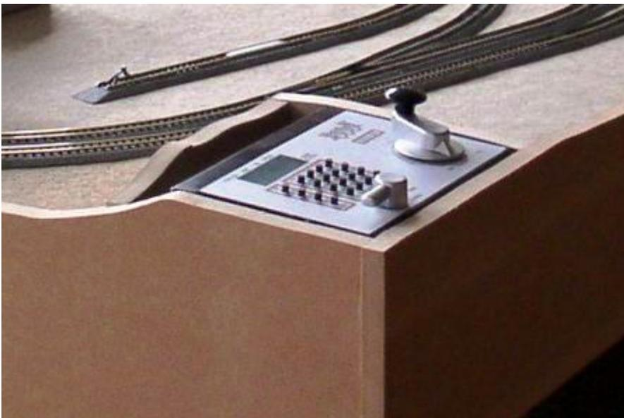
The power bus connects the terminals of the DCS50 Zephyr to the tracks of the railroad and the stationary decoders that are used to operate the track switches.
