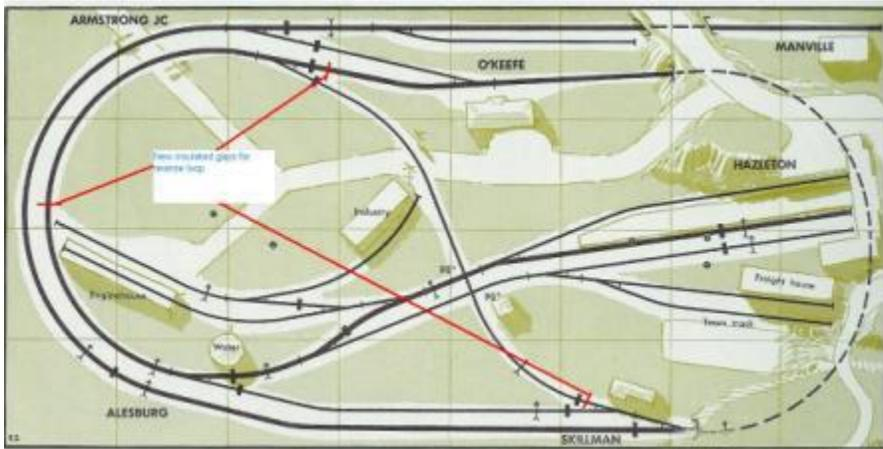
Because of the automated feature of the AR1, it does not matter if a train operating on the regular portion of the oval (from O'Keefe to Skillman) has to pass through the reversing area. The train operator never knows that the AR1 is in operation.
