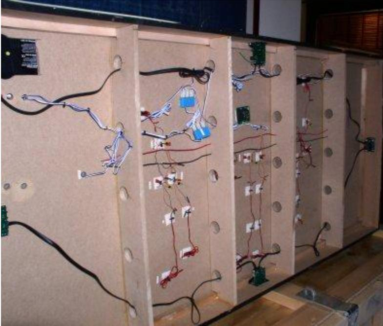
In this bottom view, the blue/white cables are the power bus cables coming from the Zephyr (*upper left*). As noted in other text, these cables have been split into groups should it later be necessary to subdivide the railroad to add an additional power booster and power supply. In the middle of the railroad is a smaller power bus which uses red and black wires; the stationary DS51K1 decoders are attached to this bus.
