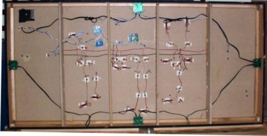
Initially, seeing all these wires can be intimidating, but as you will note, they have been grouped and bundled so that identifying the individual wires is easy. There are two groups of wires under the railroad; one group, the *power bus*, delivers power to the tracks and to the stationary decoders that operate the track switches. The other group of wires is the black cable for *LocoNet* and its devices.
