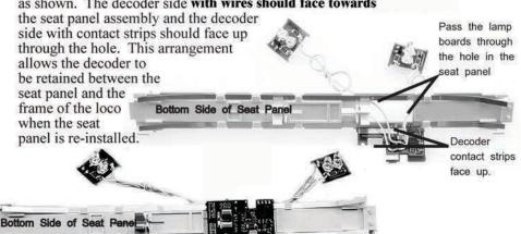
6. Carefully re-install the seat panel making sure that all brass contacts are in their
