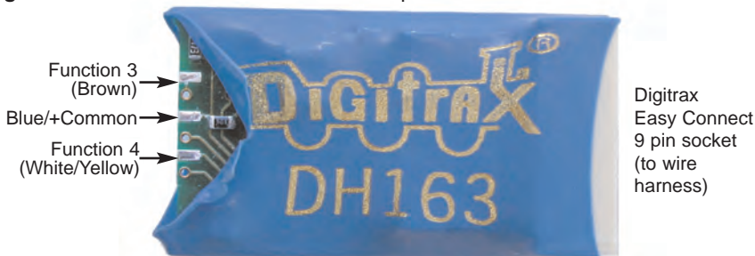
Figure 2. DH163AT Decoder Function Outputs
