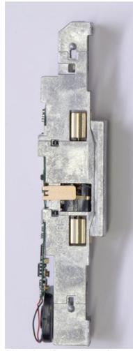
Figure 6: SD70ACE- showing a 10x18mm speaker in upper rear.
