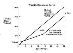
when a "straight-line" throttle response curve is used. The value of 255/xFF represents 100% motor voltage. In advanced 28/128 speed step mode, the V-start value is interpolated from the first speed step to the middle speed step or "mid" step, 15.
