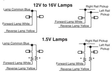
\*Note: Current setting resistor to suit the lamp used. Typically 560 ohm 1/4 watt for grain of rice and 250 ohm 1/4 watt for grain of wheat. Lower resistance values will increase the lamp brightness, minimum value is 100 ohms.
