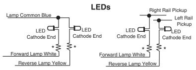
\* Note: LEDs are sensitive to polarity when hooked up. Typical resistor 680 ohm 1/4 watt.
