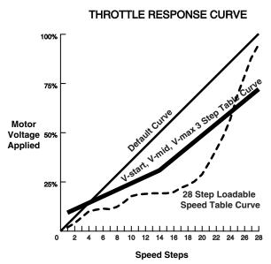
When you are using a throttle to control a locomotive, vou will notice that as you increase and decrease the speed, the loco responds to the change in throttle settings according to the relationship between motor voltage applied and the throttle setting. This is called the throttle response curve. Decoders are shipped from the factory with a linear throttle response curve. This means
