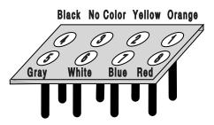
**DCC Medium Socket:** This diagram shows the DCC medium plug that is widely used with HO locomotives that come from the manufacturer with the DCC medium socket. The color code refers to the wire colors on a DCC wire harness. To install a decoder in a loco with a DCC medium socket, remove the dummy plug that comes with the locomotive and insert a decoder with a DCC medium plug in the socket.
